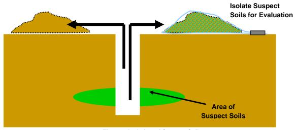
Figure 2 Isolation of Suspect Soils
